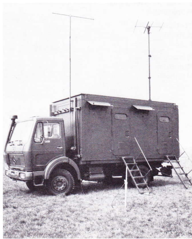
Mobile Rundfunksendestation 10 kW (MW) Mobile broadcasting transmitting station 10 kW (MW)
